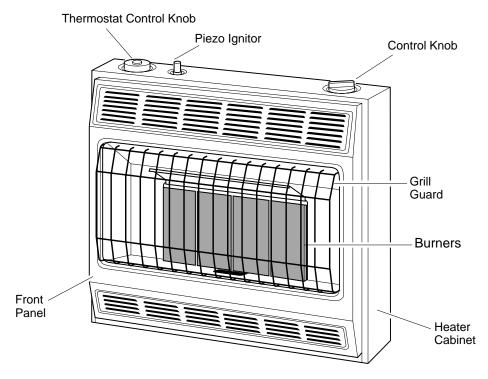
Figure 1 - Vent-Free Natural Gas Heater (Model VN2550ITB Shown)
